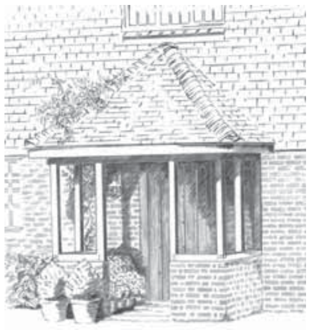
Porch in character with the house
